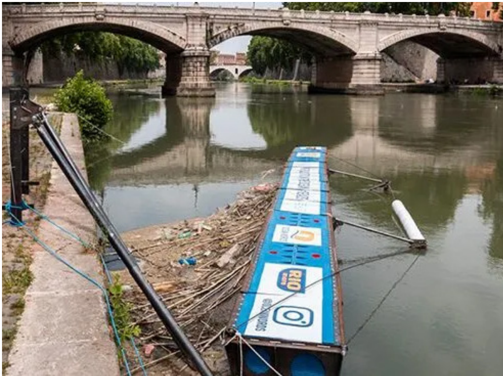
Test instalation of a trash barrier on Timber river, SEADS
