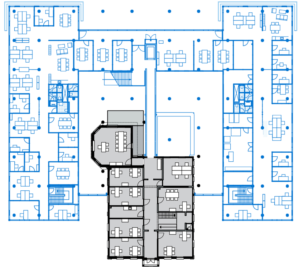
fig. 62 ground floor plan - temporary intervention in blue (source: plan by RAU Architekten, edited by Kewin Niewiarowski)
